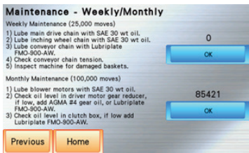
Display Of Maintenance Screen
