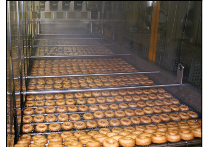
Multimatic MDDRF-8 deposits 16 mini donuts across the fryer, shown with C10-36G fryer
