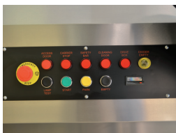
The easy to reach control panel features an integrated dough processing counter to record the number of products produced.
