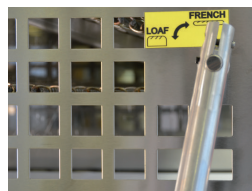
Simple to use lever to set the curling chain required for either loaves or French sticks.
