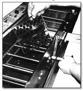
Figure 4 Removing the Turner
