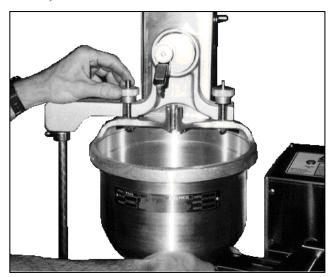
Figure 1-6. Mounting the Hopper.
