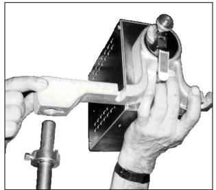
Figure 1-5. Mounting the cutter head.
