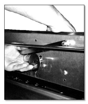
Figure 3 Removing the Turner Cam
