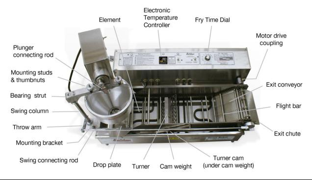
Figure 1.1. Above: Donut Robot Mark II. (components apply also to Donut Robot Mark V)
