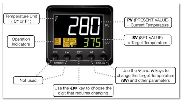
Figure 1.2, Temperature controller
