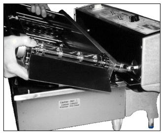
Figure 1-2. Joining the Couplings.
