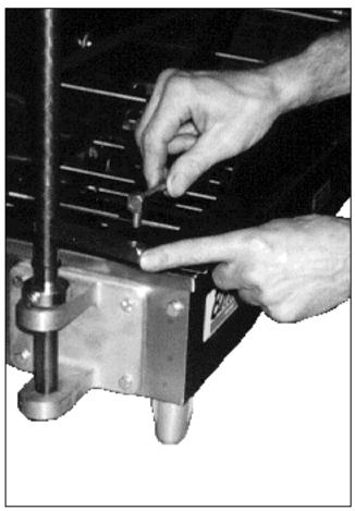
Figure 1-4. Connecting the Swing Connecting Rod.
