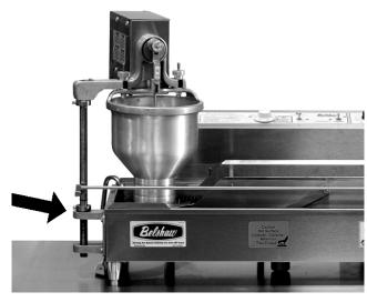
Figure 2-2. Lubricating the swing column.
