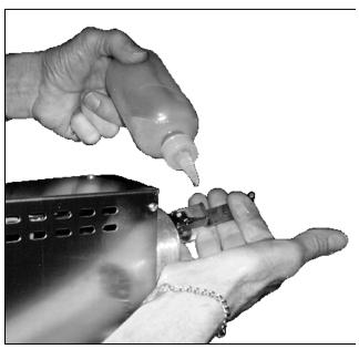
Figure 2-1. Lubricating the Connecting Rod.
