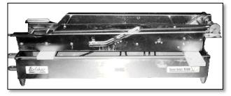
Figure 2: Rest the conveyor on the fryer.
