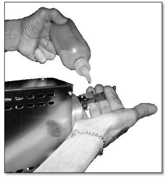
Figure 6 Lubricating the Connecting Rod.
