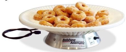
The Roto Cooler is designed to catch and cool donuts as they drop from the outfeed end of the Donut Robot.
