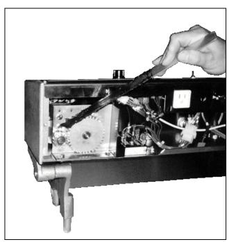
Figure 2-3. Lubricating the Drive Gears.
