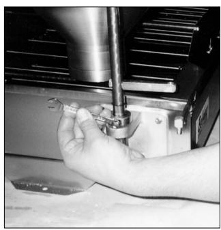
Figure 1-8. Adjusting the Height of the Hopper.
