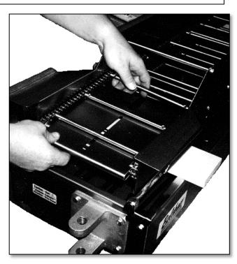
Figure 5 Removing the Drop Plate
