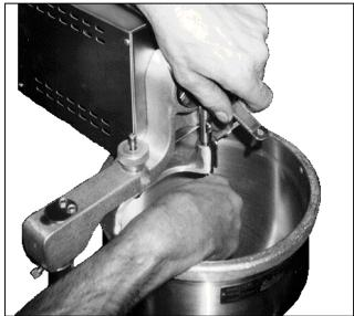
Figure 1-7. Installing the Plunger.
