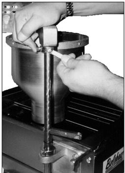
Figure 1-9. Adjusting the Swing of the Hopper.
