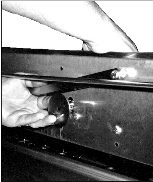
Figure 3 Removing the Turner Cam
