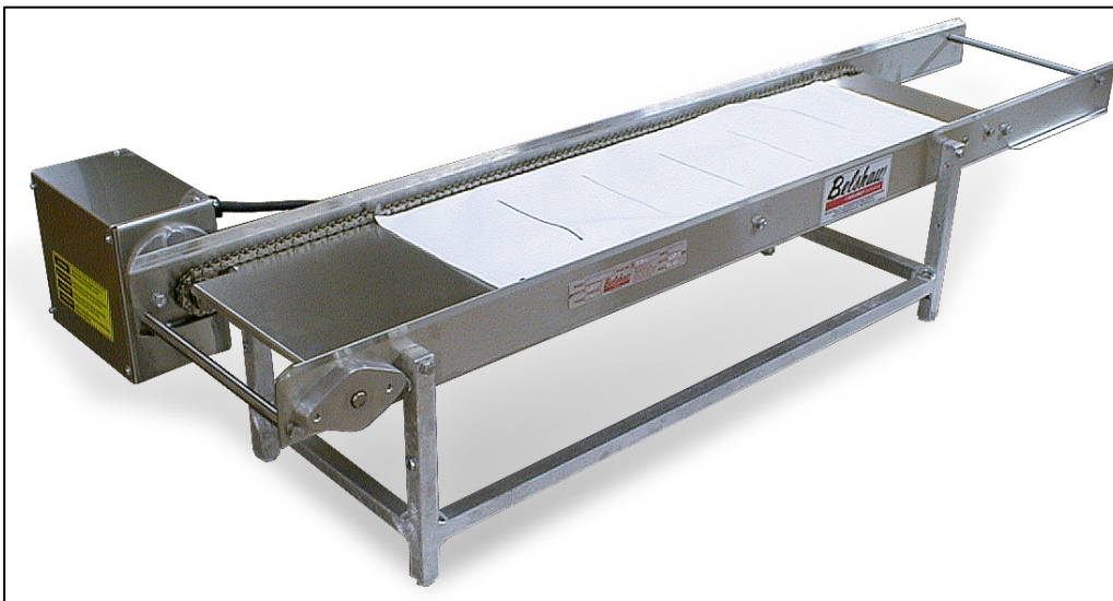
Figure 7 FT-42 Feed Table with Feed Table cloth.
