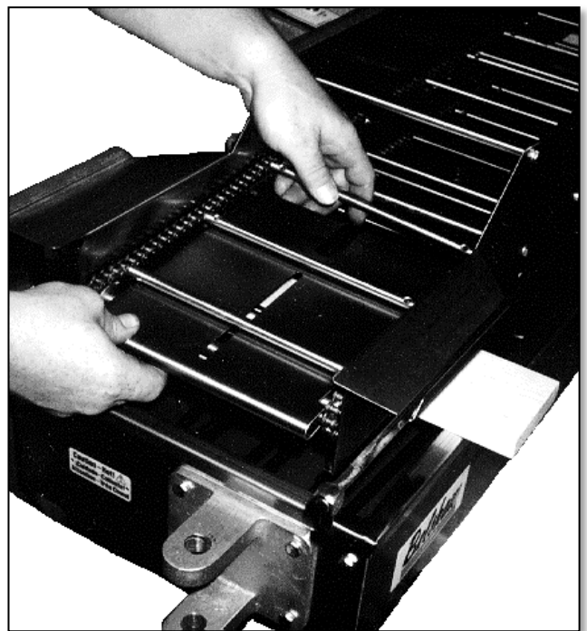
Figure 5 Removing the Drop Plate
