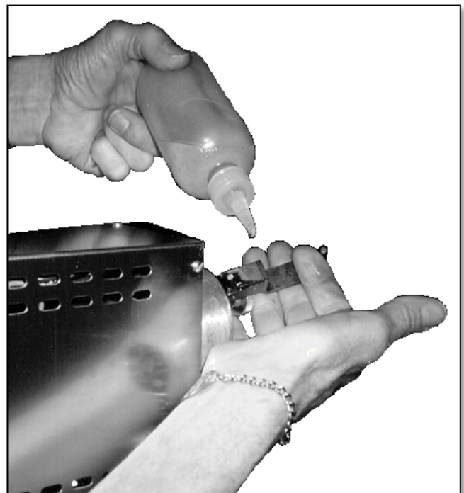
Figure 6 Lubricating the Connecting Rod.
