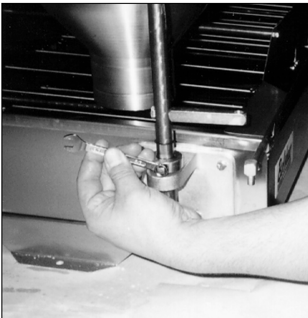
Figure 1-8. Adjusting the Height of the Hopper.
