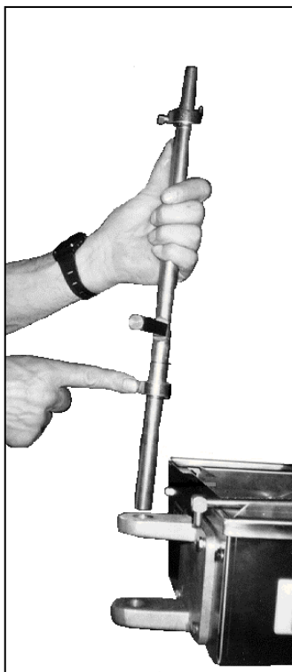
Figure 1-3. Inserting the Swing Column.
