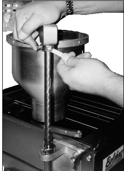
Figure 1-9. Adjusting the Swing of the Hopper.
