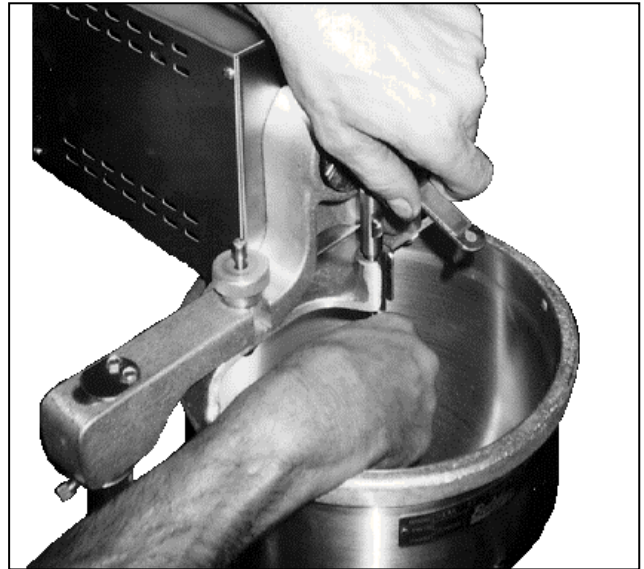
Figure 1-7. Installing the Plunger.
