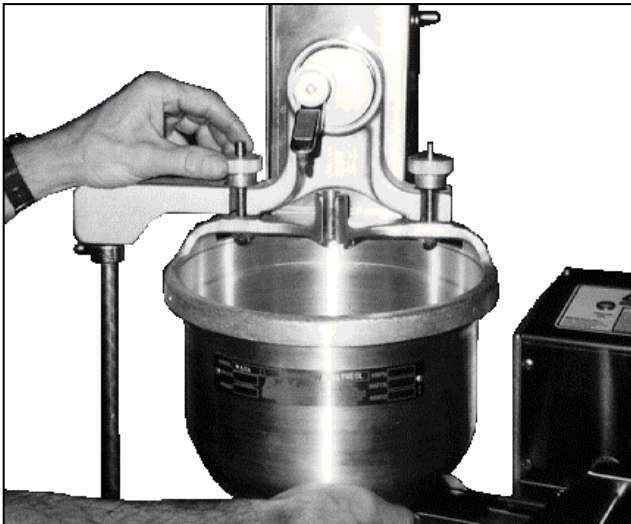
Figure 1-6. Mounting the Hopper.
