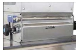
Centrally adjustable infeed flaps in hopper with size indicator
