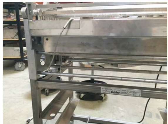
Figure 6, Installation of Thermocouple
