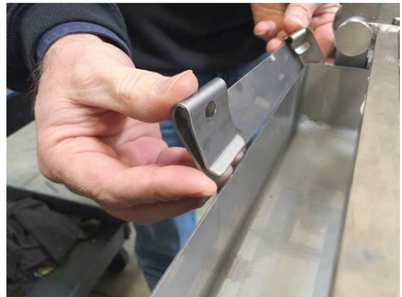
Figure 5, Installation of Thermocouple Bracket
