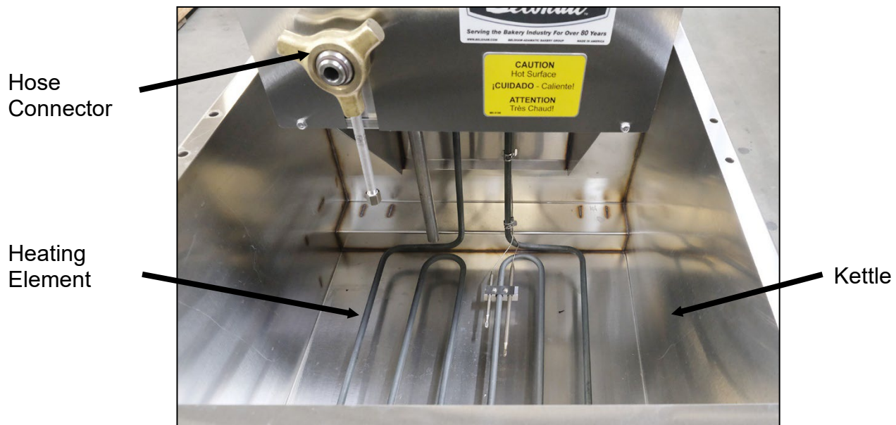
Figure 1-3. Top View, Kettle and Elements (with Cube Melter removed).
