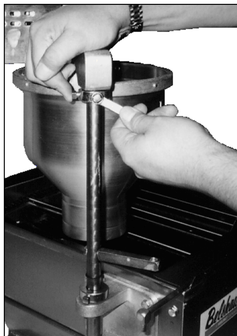
Figure 1-9. Adjusting the Swing of the Hopper.
