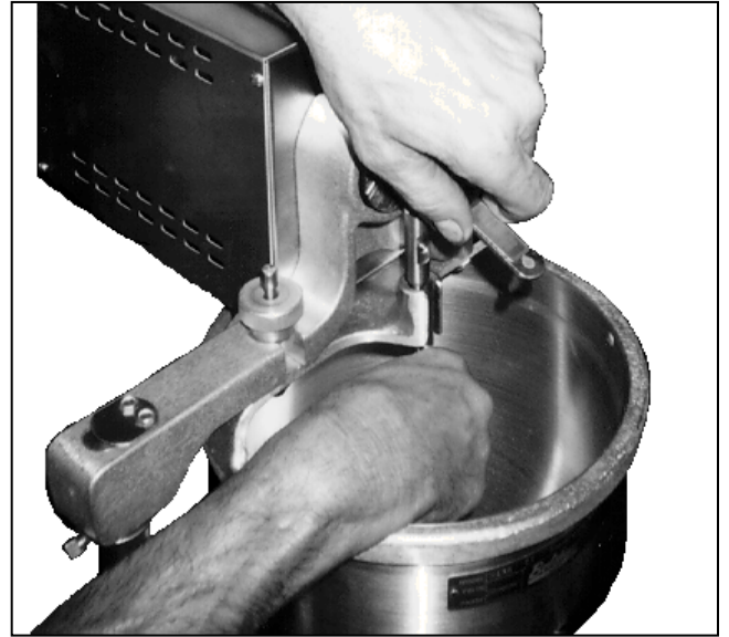
Figure 1-7. Installing the Plunger.
