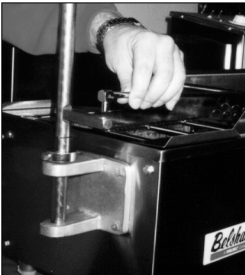
Figure 1-4. Connecting the Swing Connecting Rod.
