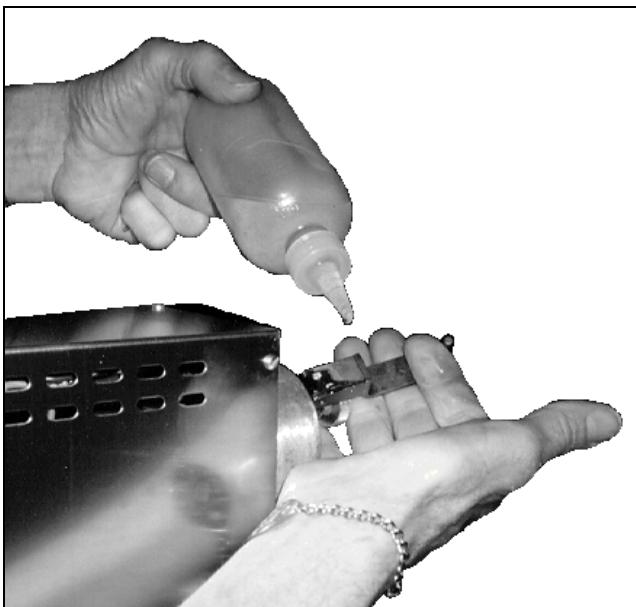
Figure 2-1. Lubricating the Connecting Rod.
