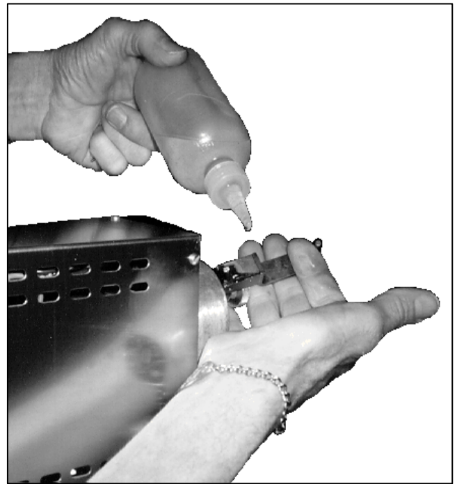
Figure 4-1. Lubricating the Connecting Rod.
