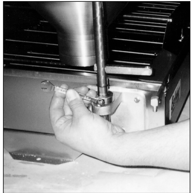
Figure 1-8. Adjusting the Height of the Hopper.
