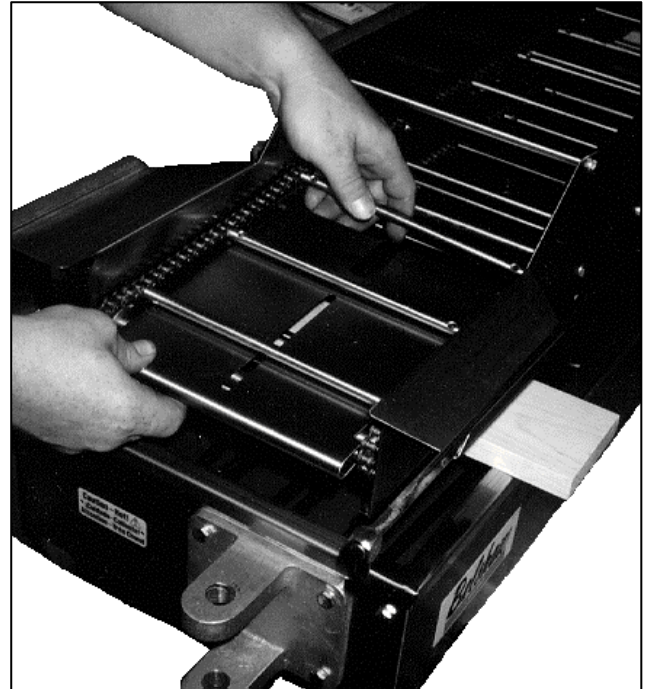
Figure 3-4. Removing the Drop Plate.
