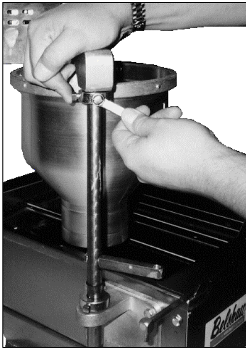
Figure 1-9. Adjusting the Swing of the Hopper.
