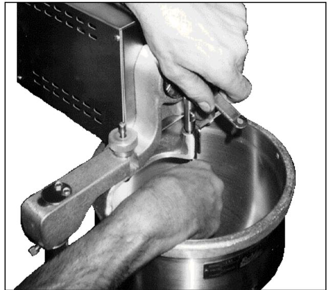
Figure 1-7. Installing the Plunger.
