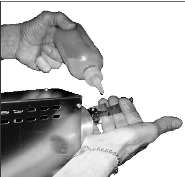
Figure 2-1. Lubricating the Connecting Rod.
