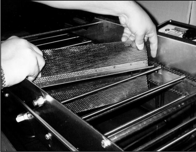
**Figure 4 Removing the Turner**
