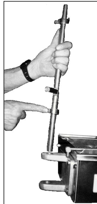
Figure 1-3. Inserting the Swing Column.
