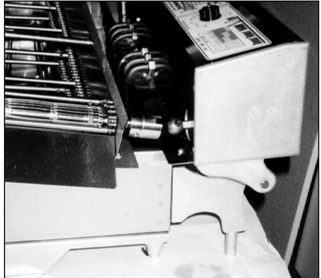
Figure 1-2. Joining the Couplings.
